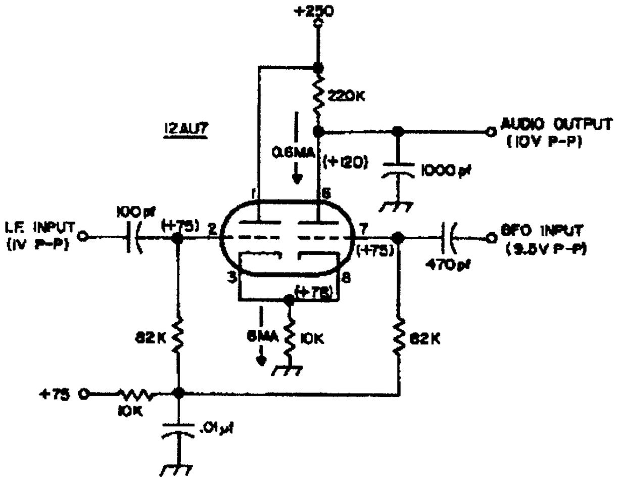
**Fig. 1. Modified Like New mixer circuit.**
