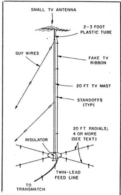
Fig 6—WB6AAM's antenna can be camouflaged easily as a commercial-TV installation. (For clarity, only one set of guy wires is illustrated.) [One could eliminate the top plastic tube and bond the TV antenna to the mast top as capacitive loading. This would make the antenna electrical length slightly longer than 20 ft.—Ed.]
