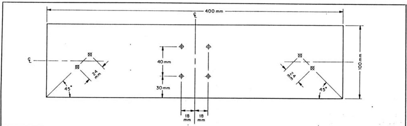
Fig 2—Drilling pattern for the mounting plate. [Dimensions are in mm; inches = mm  $\times$  0.0394. Size holes and adjust locations to fit locally available hardware. The mounting plate may be hardwood rather than plastic, or plastic sleeves may be used to insulate the elements from a metal plate if a plastic plate is not available.—Ed.]
