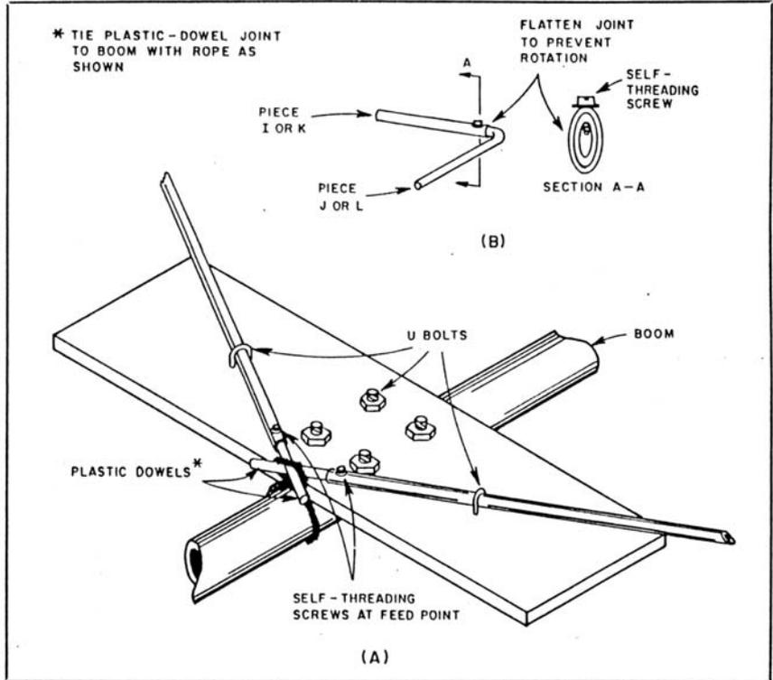
Fig 3—Details of the mounting-plate assembly (A) and element joint (B). Flatten the joint slightly after assembly to prevent rotation.
