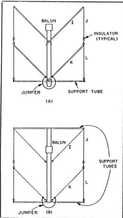
Fig 4—Variations on the Sigma beam that increase strength by reducing weight and mechanical complexity. Wire is used for the element end sections at A, while all conductors are wire at B. Wire lengths are the same as the tube lengths given in Table 1.
