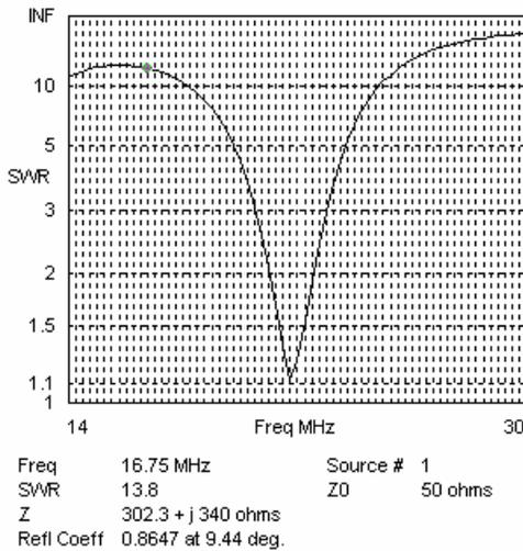
SWR plot of bottom fed single wire, 10 metres long, with base 0.5m above average ground – this is off the scale due to reactive impedance being in the tens of thousands of Ohms. Even over salt water, the SWR plot is the same. Obviously it will match but how efficiently? Will the losses in the tuning circuit be much higher due to the far greater impedance mismatch?
