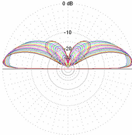
Now, the same sweep for a 10m tall bottom fed vertical. Note that from 17MHz upwards the angle of radiation increases rapidly. On the higher frequencies from about 22MHz there is very little low angle radiation. The only way to keep the radiation angle low is to shorten the antenna with each band change.
